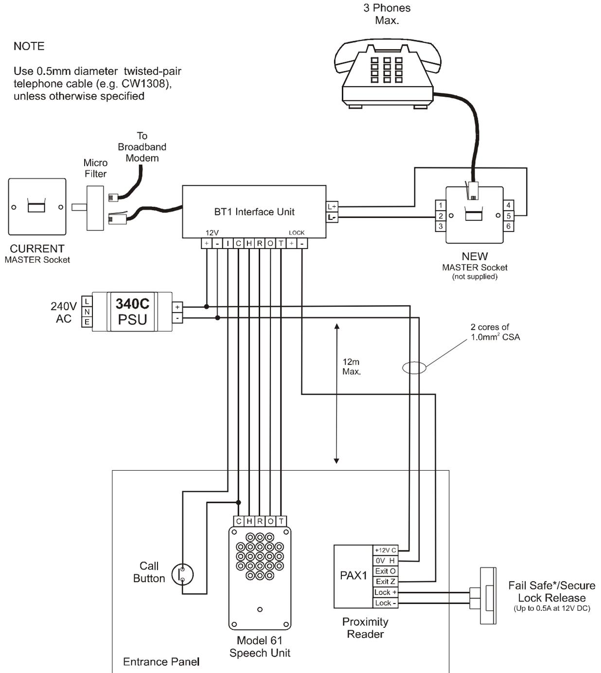
**\* If a Maglock is used, a suitable transient suppressor must be fitted directly across the Maglock.**
